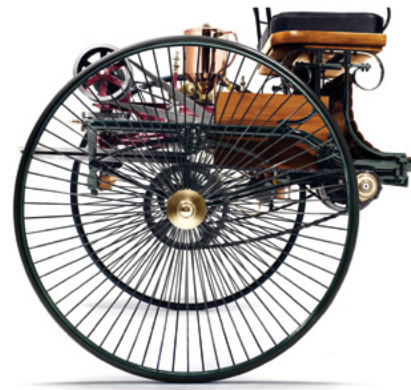
FIGURE 1 The Patent Motor Car developed by Carl Benz in 1886 was the first car with a combustion engine; it was driven by a belt transmission (© Mercedes-Benz Classic)
